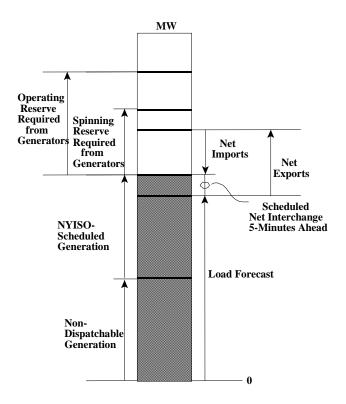
Figure 22: Control Area Constraints
